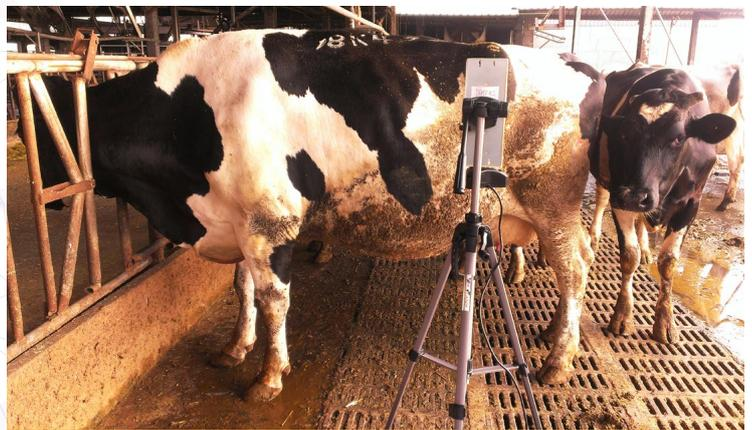
Touch-less monitoring of cow's vital signs using SIL Doppler radar
